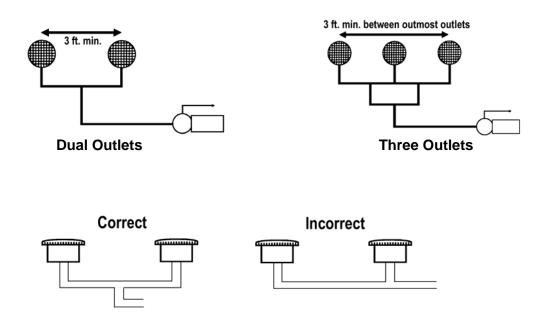
b. Each branch of a split suction shall terminate under its own suction outlet cover/grate. Except, suction plumbing from two different pumps may terminate under one suction outlet cover/grate if the combined flow rate of each suction pipe is less than the flow ratings of a single cover/grate.
